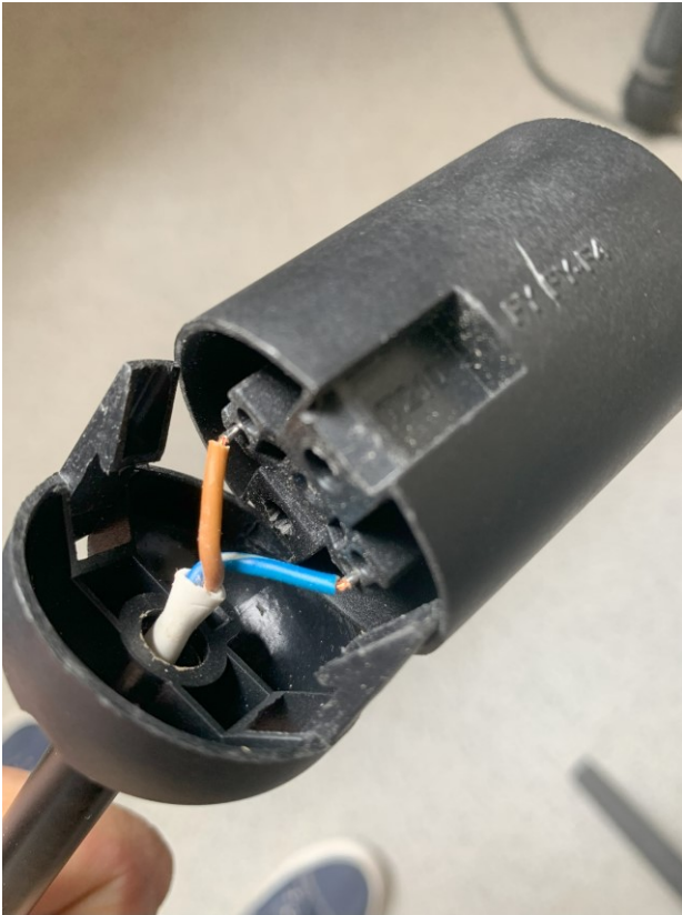
Disassembled view of the lampholder, power supply connection
