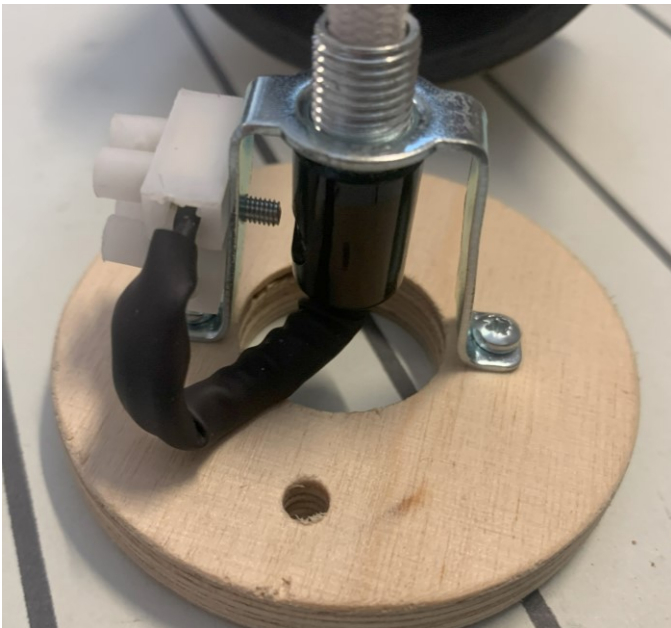
Terminal block and suspension cord fastening
